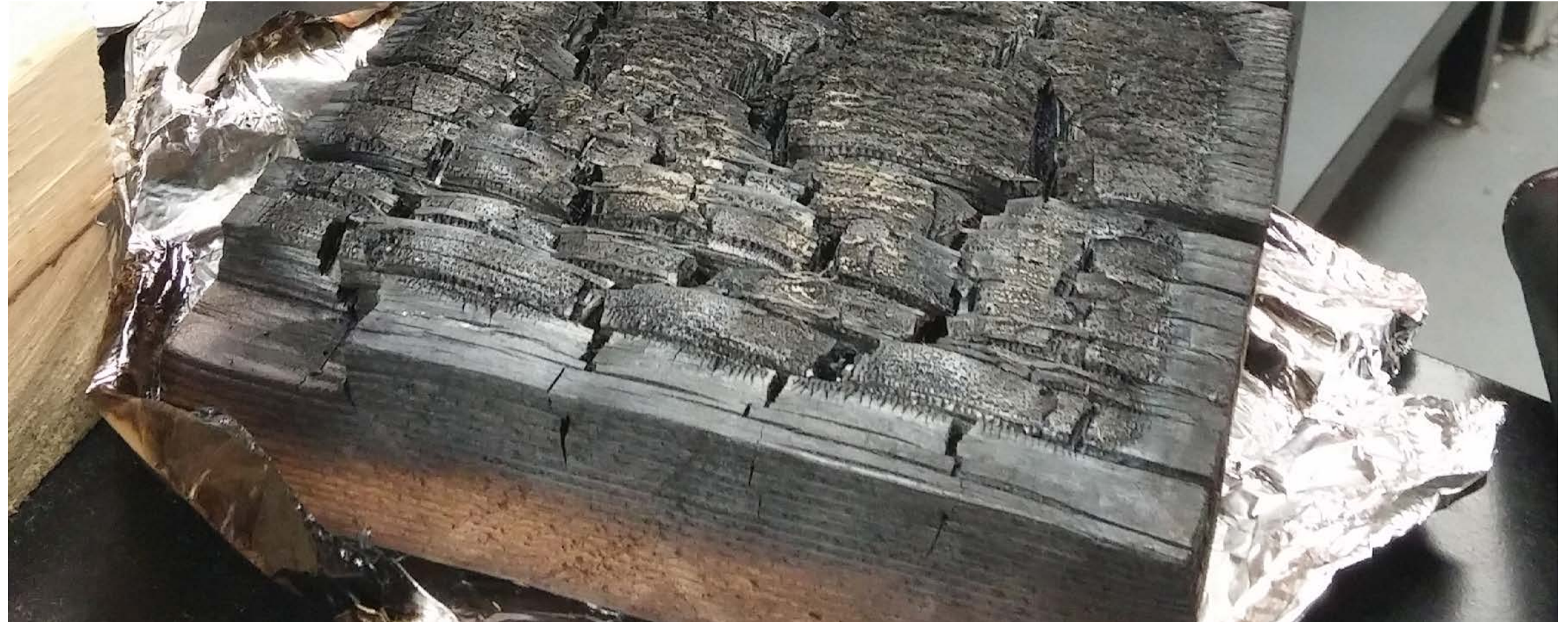
Figure 3.4 Wood charring Photo courtesy of Holmes Fire
