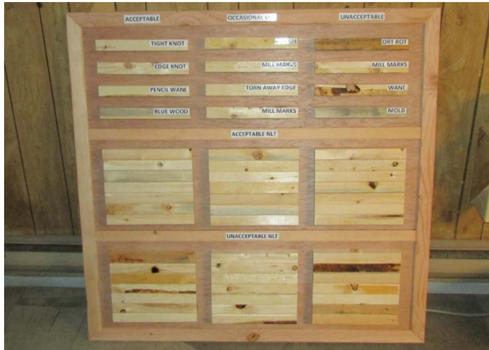
Figure 6.2 Example of aesthetic grade boards for NLT panels Photo courtesy of StructureCraft
