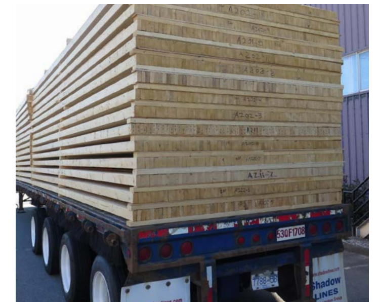
Figure 8.1 Shipping with dunnage and stickers Photo courtesy of StructureCraft
