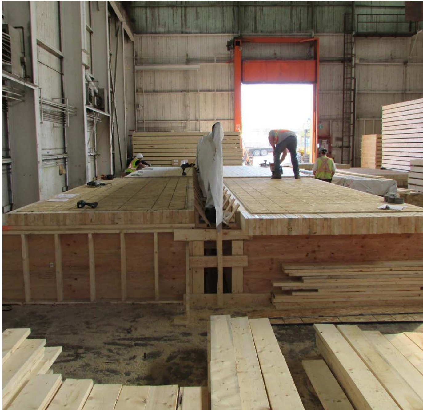
Figure 7.3 NLT fabrication setup Photo courtesy of StructureCraft
